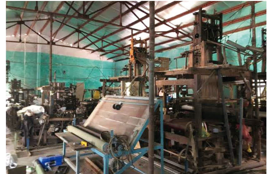
The above is a wooden textile weaving machine that was being used to produce silk fabrics locally. It had problems in production efficiency, production diversity and durability.
