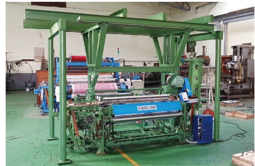
The above is a new silk weaving machine made by Sambo Engineering. Productivity increased by 30 ~ 40% compared to the conventional wooden weaving machine and work efficiency increased by installing an automatic detection system.
