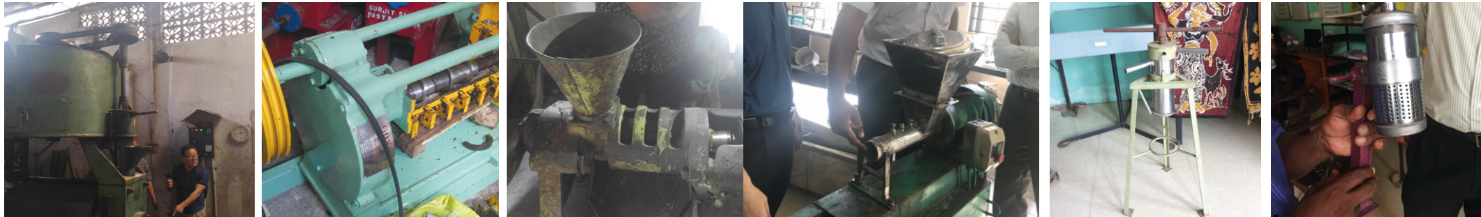
Starting from the left, large-sized oil extractor from India, medium-sized extractor from China and small extractor from Sri Lanka. They are all made of cast iron so, heavy, vulnerable to humidity and easy to rust.
