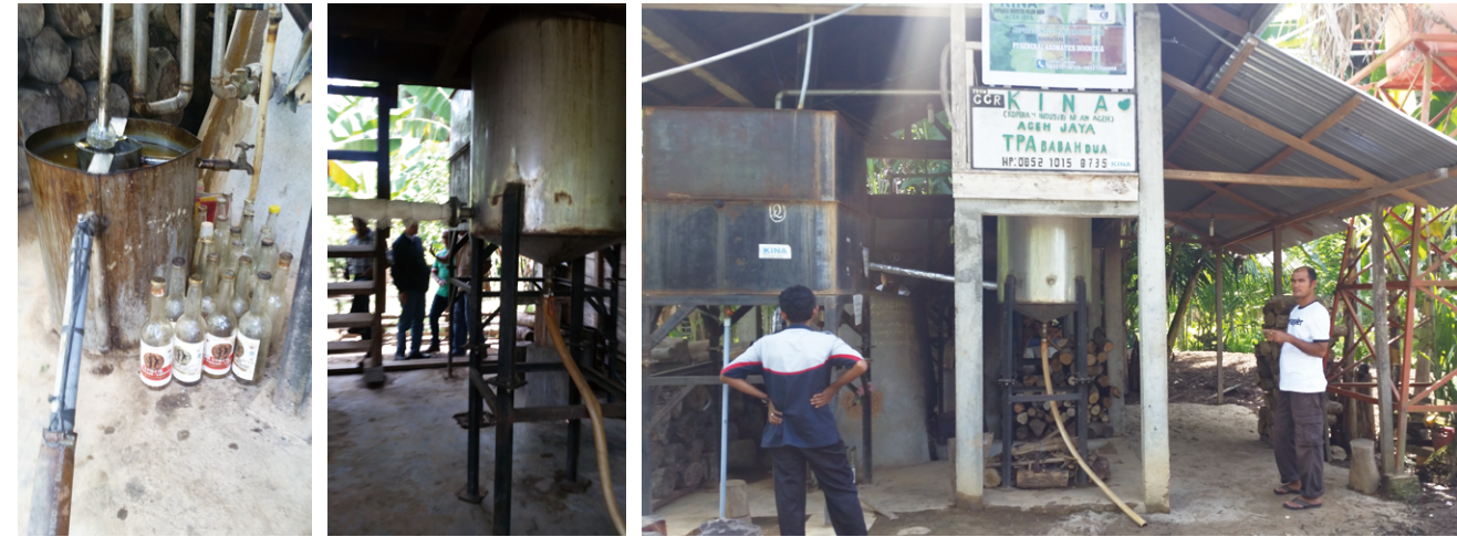
Traditional extractor had issues in its low work efficiency from the poor structure and low production quality from corrosion.
