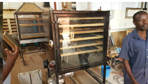
From the left, a dryer developed by Makerere University and various dryers used in Uganda. They had issues in the capacity, durability and usability and they were unable to cater for locals' needs.
