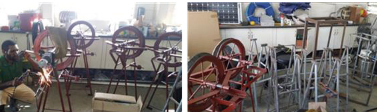
One of the engineers from NARI is making a rope pump after AT production training by an expert from Korea
